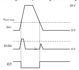
Figure 16. Overvoltage Protection Waveform, 20 V
