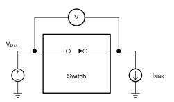
Channel ON,  $R_{ON} = V/I_{SINK}$
