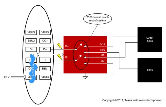
Figure 15. Protecting During a 20-V Short
