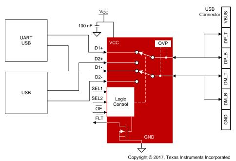
Figure 17. Typical TS5USBC402 Application
